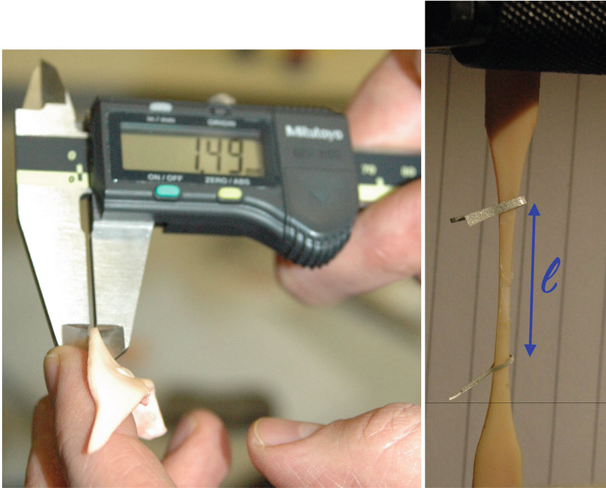
Fig. 3.7 Left: Measuring the reference cross-sectional dimensions of a sample with a Vernier calliper. Right: Clamping the sample in a tensile machine and tracking the current length \ell using two reflective markers, with positions tracked by a vertical laser beam
