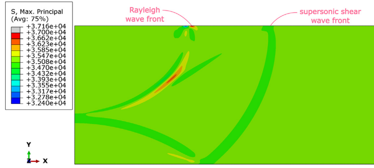
Fig. 6. Maximum principal stress (Pa) in the deformed neo-Hookean material with a Young's modulus of 175 kPa, a density of 1,116 kg m -3 and a pre-stretch of 1.2 (20% extension). This frame of the simulation was taken after 0.553 ms of wave propagation. The (larger) Rayleigh wave can be seen travelling along the surface of the skin, as well as the faster supersonic shear wave.
