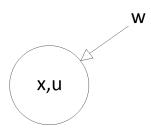
x is the internal temperature w is the external temperature u is the thermal power
