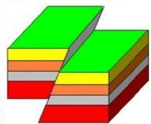
When the applied force is too big an earthquake occurs. The segments slide over each other until they reach a new configuration.
