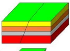
In static conditions the segments are sticked. The strain makes to increase the applied force that is counterbalanced by the dry friction between the contact surfaces.
