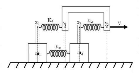
The system can be modelled as a 2-DOF mechanical system.
