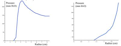
He also tested a monkey bladder (right). In this case, the pressure-stretch curve exhibits monotonic increasing, exponential-like behaviour.
