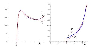
The Gent model provided the best fit for the rubber balloon, while the Mooney model provided the best fit for the bladder. However, the bladder is highly anisotropic so this model may be inadequate.
