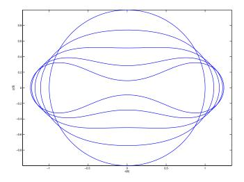
Figure: Cross sections of the axisymmetric deformation for p = 6.0 (spherical), 6.5, 7.0, 7.5, 7.9; deformation increases with pressure
