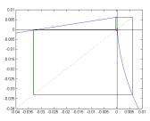
A grazing bifurcation is an effect of the fact that an impact with low velocity is sensitive to small changes in the initial conditions, with sensitivity inversely proportional to impact velocity.
